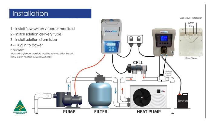
Next, connect the solution drum to the left hand nipple of the peristaltic pump.
